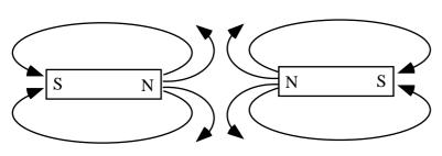
can be easily observed using iron filings and two bar magnets. These diagrams clearly show that opposing flux lines result in attraction, while unidirectional flux lines from different sources result in repulsion.
