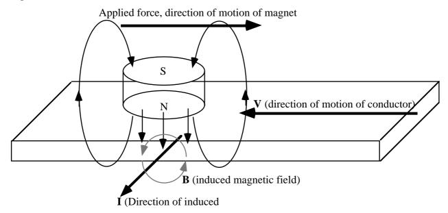
It is important to realise that the current is induced in the conductor and not in the magnet, therefore it is the relative direction of motion of the conductor which must be considered. An opposing (attracting pole) will form on the surface of the conductor near the leading edge of the magnet, relative to the direction of motion of the conductor, as shown in the diagram below.
