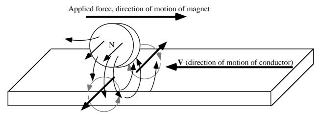
Again it can be seen that there is an attraction at the leading edge of the magnet and a repulsion at the trailing edge. However, as only a very small proportion of the flux lines will interact with the conductor, the resulting forces from this interaction are minimal, as an experiment will confirm.
