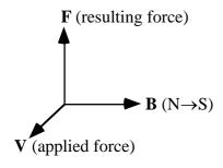
For a conductor carrying a current,  $\mathbf{B}$  is the direction of an external magnetic field,  $\mathbf{V}$  is the direction in which the conductor is pushed, the direction of motion, and  $\mathbf{F}$  is the direction in which the electric current (positive charge) is induced. This is true for any conductor in relative motion perpendicular to the direction of any magnetic field.
