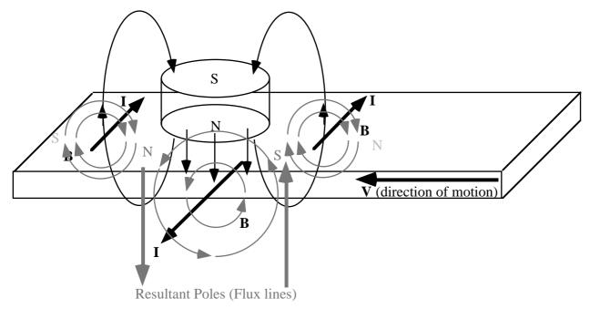
It is important to note that if the magnet were placed upside down (South face down), all flux lines, poles and directions of currents would be reversed, but the resulting forces would be the same, that is attraction at the leading edge and repulsion at the trailing edge.
