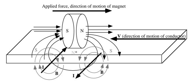
Of the three induced poles, the  $\mathbb{N}^*$  is in an area where the magnet has no or very low flux density hence the induced  $\mathbb{N}^*$  pole will have no affect on the resulting forces experienced by the magnet held in this position and moved along the conductor. The two induced  $\mathbb{S}$  (south) poles, have the affect of attracting the leading edge of the magnet and repelling the trailing edge of the magnet.
